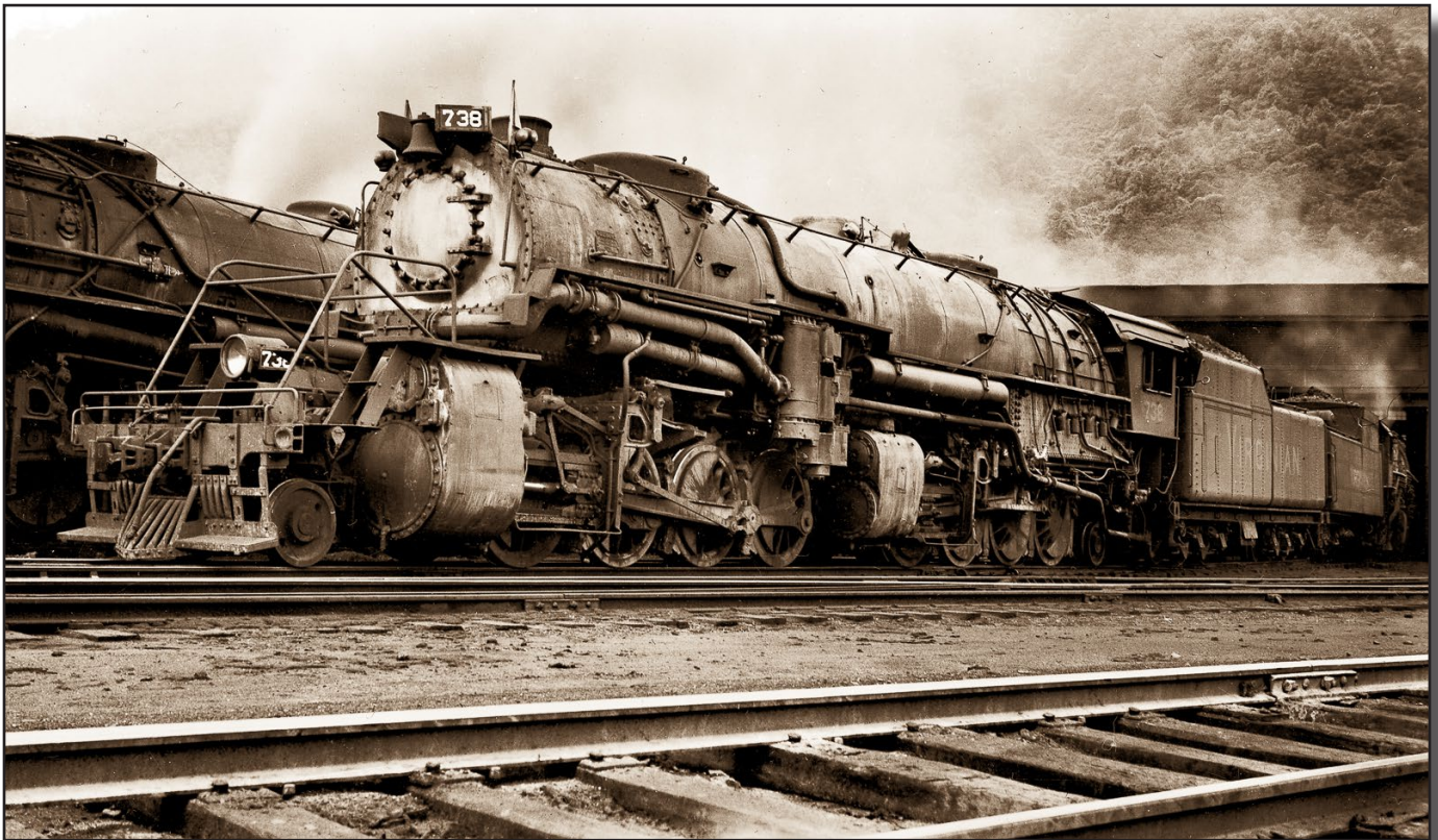
Virginian Railway 738 is steaming up at the engine facilities at Elmore, WV on April 4th, 1950. The 2-8-8-2 was built by ALCO-Schenectady (c/n 61090) in 1919. Scrapped in June of 1955. Donald R. Hensley, Jr. Collection (616 size negative) Original photographer unknown.
