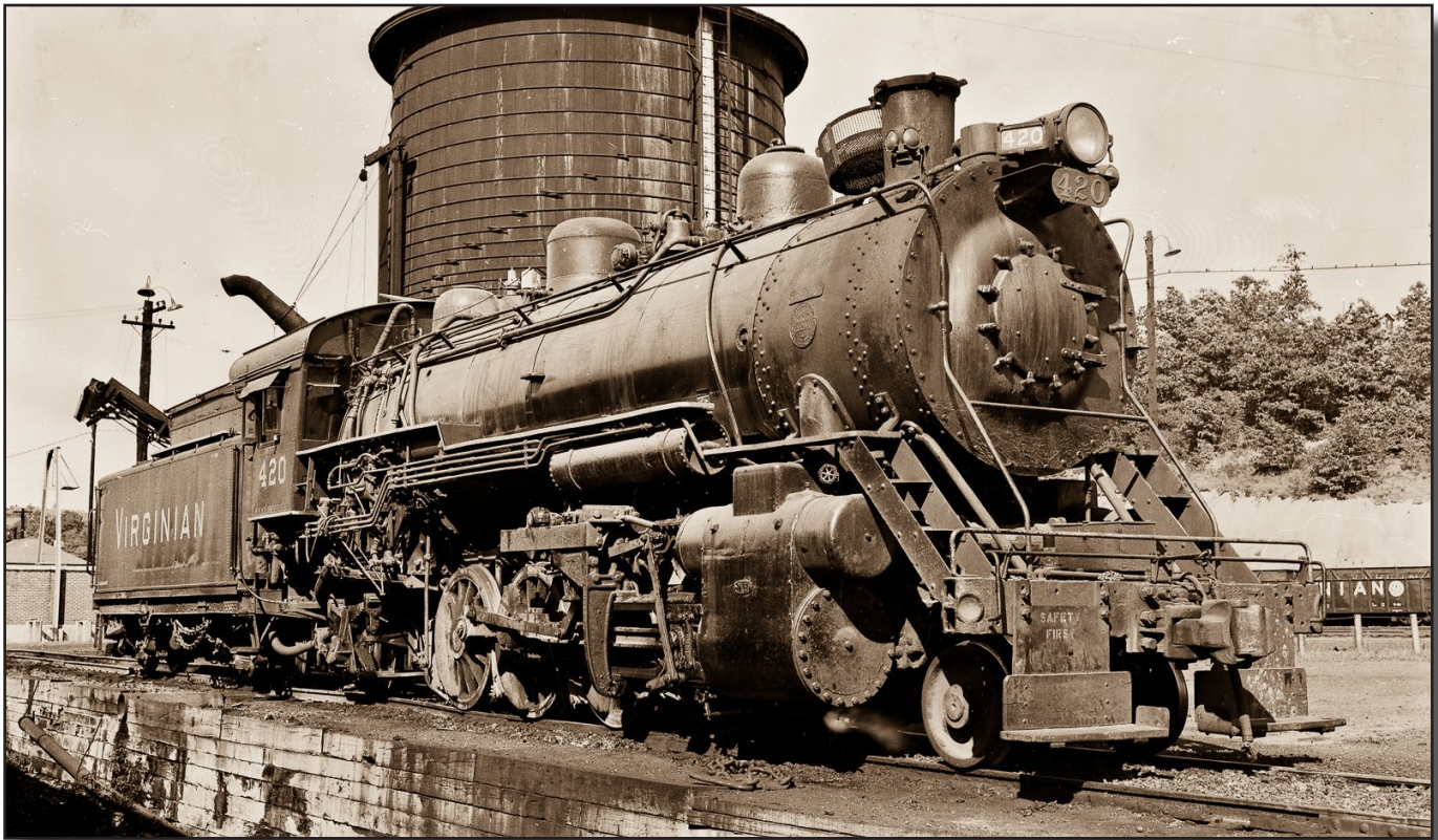
Virginian Railway 420 taking on water at Princeton, WV on September 5th, 1954. This Mikado was built by Baldwin (c/n 33395) in 1909 and would be scrapped in March of 1955, only six months away. Donald R. Hensley, Jr. Collection (616 size negative) Original photographer unknown.
