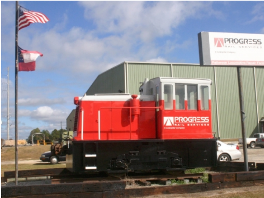
Progressive Rail's critter has been used to move engines around the shop.
