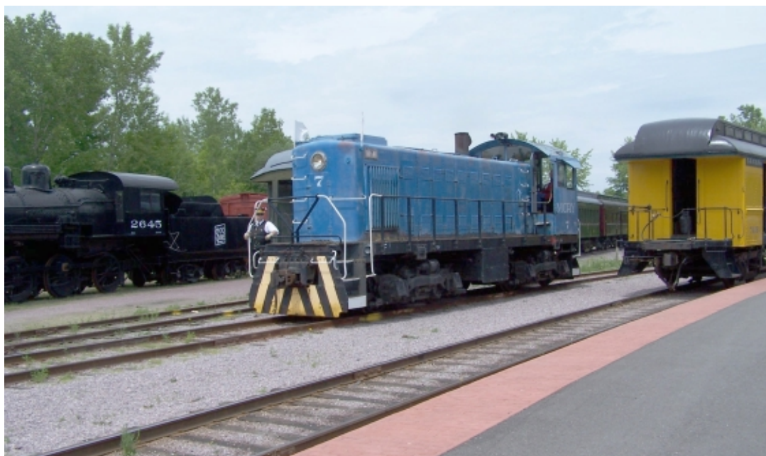
The motive power for today’s train was engine No. 7, a 69 year old Alco S-1 built in 1944.
