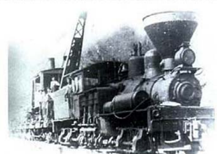
The single locomotive for Moltz Lumber Company was a Shay, shown above with a log loader. Courtesy of the U.S. Forest Service.
