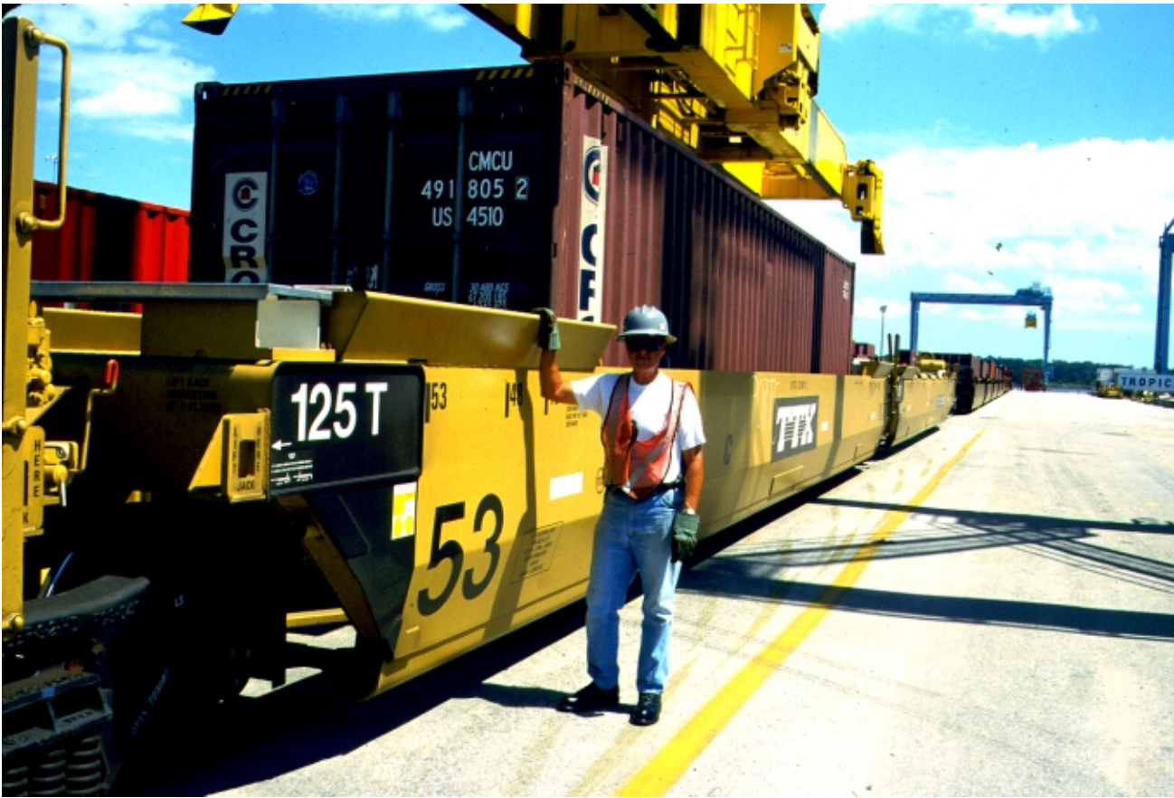
Jim Smith standing in front of a double stack illustrating how high the walkway is that you must use to place or remove a locking pin.
